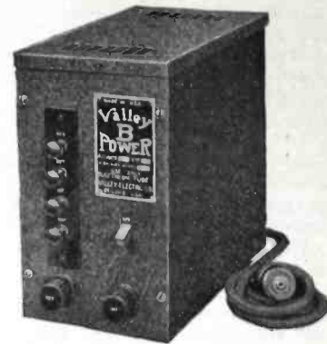
The Valley B power unit provides adjustable voltages to suit the requirements of any receiver.
